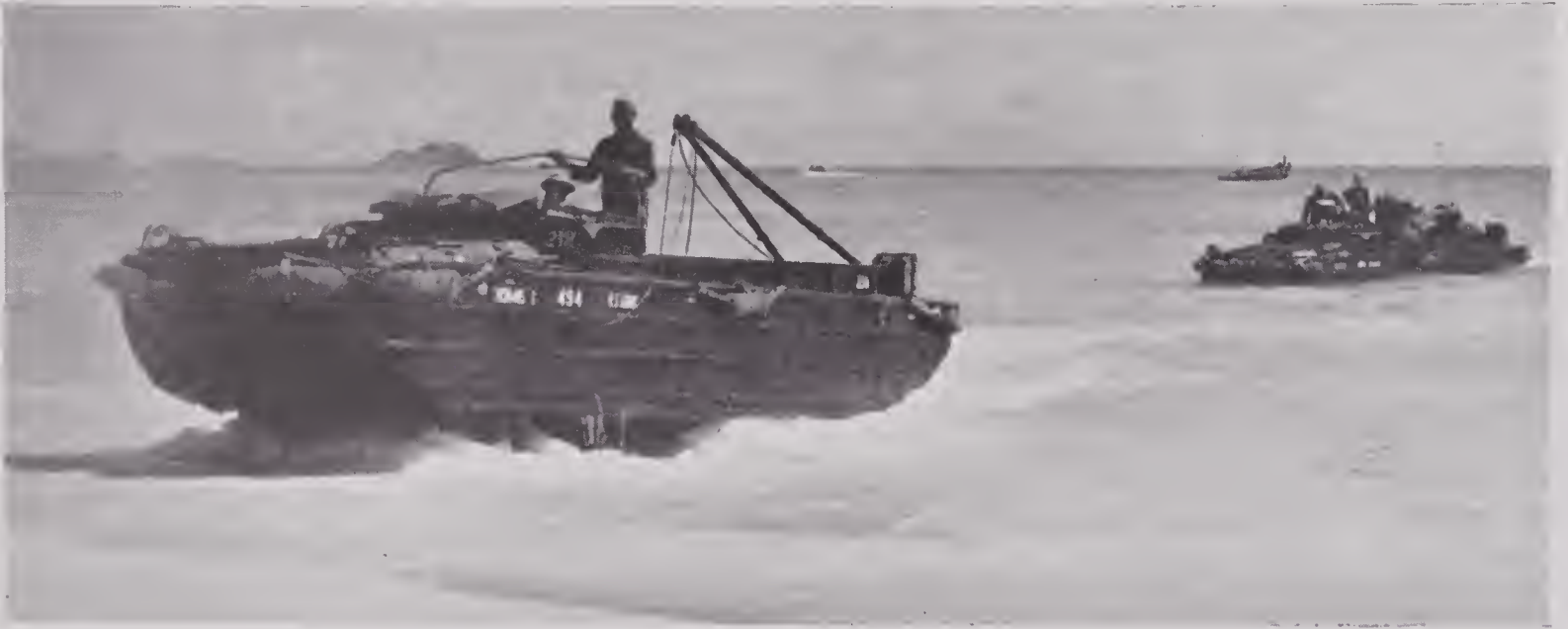
FIGURE 3. DUKW drivers in training at Waimanalo school, Oahu, transporting 105-mm howitzer. A-frame DUKW leads way to beach so A-frame can be set up by time howitzer arrives on shore.
